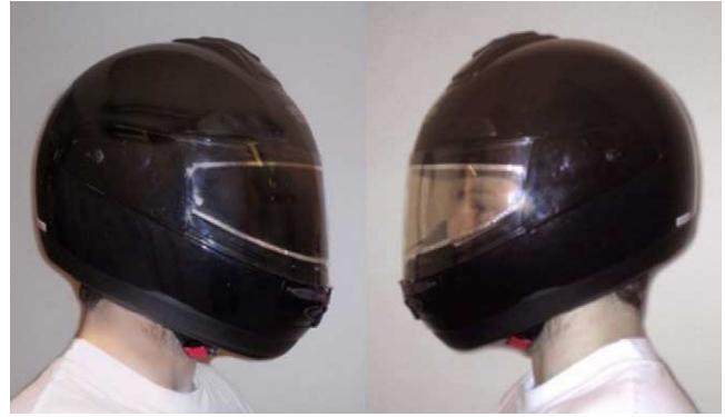
Fig. 11. Electrochromics-based variable-transmittance visor for safe motorcycle riding.
